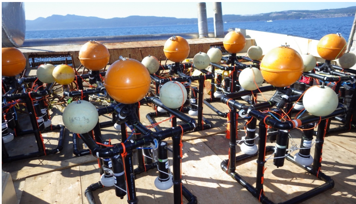
Figure 7. Malaspina Strait sub-array moorings equipped with amplified and unamplified 69 kHz VR2 receivers, and amplified and unamplified 180 kHz VR2 receivers. The ABS frames are designed to flood and be almost completely transparent to sound.
